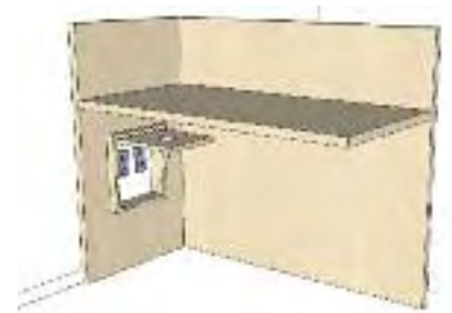
R10 Modesty Panel Receptacle Access Flap hinged flap permits access to a wall outlet through an end panel or modesty panel.
